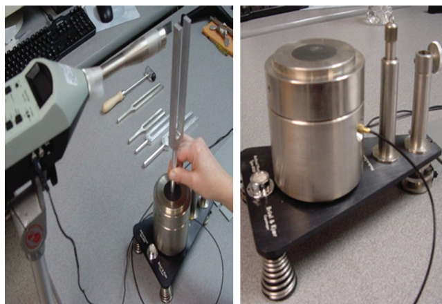
Figure 2. Setup for simultaneous measurement of air and bone conduction. Left: Tuning fork being applied to membrane of artificial mastoid. A ruler was used to control the distance (1 cm) between the microphone and the nearest tine across forks. Right: Close-up view of artificial mastoid.
