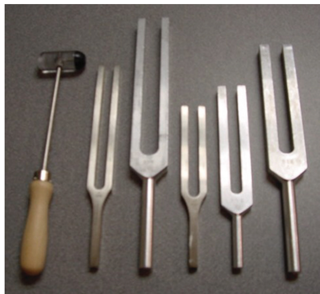
Figure 1. Tuning forks used to measure relative bone/air conduction. From left to right, mallet used to strike the forks, 256-Hz steel, 256-Hz aluminum, 512-Hz steel, 512-Hz aluminum (standard), and 512-Hz aluminum (large).
